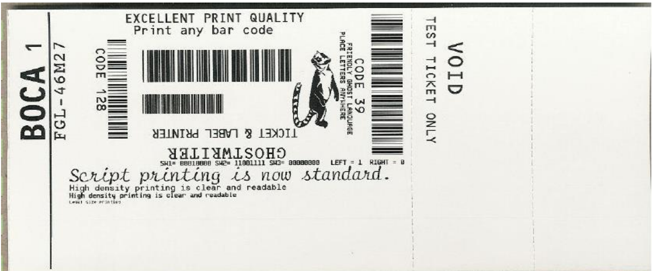
Above sample FGL ticket was printed on a 3.25" x 8" (receipt) ticket using a RADJW-3.25 200dpi FGL printer
