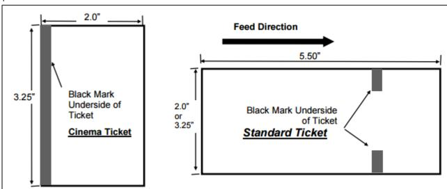
When loading 5.50" long ticket stock the black timing mark should be closest to the leading edge of the ticket (the first part that goes into the printer). When loading 2.0" long cinema ticket stock the black timing mark should be furthest away from to the leading edge of the ticket (the first part that goes into the printer).
